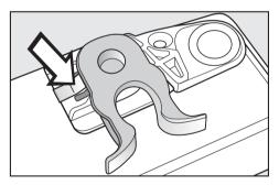
Using a screwdriver, remove spring clamp <sup>(3)</sup> from underneath the door and fit it on the opposite side.
